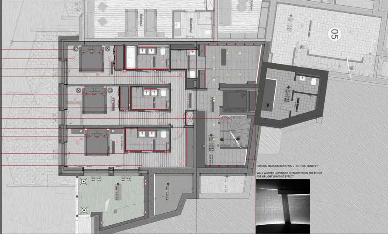
NATURAL RANDOM ROCK WALL LIGHTING CONCEPT: WALL WASHER LUMINAIRE INTEGRATED ON THE FLOOR FOR UPLIGHT LIGHTING EFFECT
